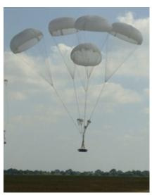
fabric for P7 heavy cargo parachutes. Kusumgar successfully developed the fabric with special coating formulation with the support of DRDO's ADRDE team, which resulted in
